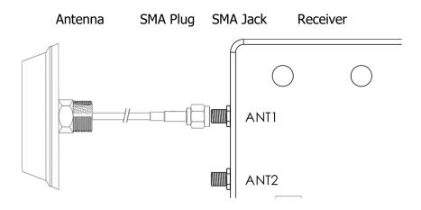
The cable connected to the antenna needs to be cut to a manageable length of 15 cm [6 inch] and a SMA Plug needs to be soldered and crimped. The core has to be soldered to the pin. Then slide the metal sleeve with the cable's shield over the back of the connector and crimp them together. Measure between the pin and the shield to make sure they are isolated from each other (i.e. not electrically connected).
